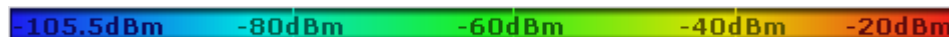
Fig. 4-14: Linear color curve shape = 0; colors are distributed evenly over the complete result range
